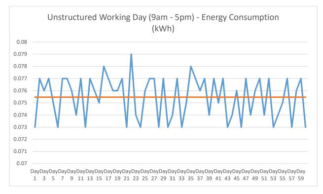
Figure 1 – EUC device daily electricity consumption when operated 9am to 5pm in an unstructured manner
